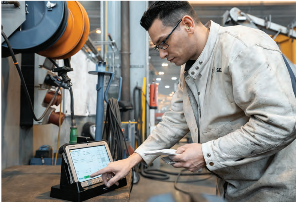
The ViWIS assistance system merges information from different systems. Workers log on to the portable operational data acquisition system (BDE) on their tablets with their employee card at the start.
