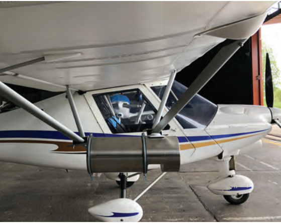
The aerial scanner is mounted on the light aircraft's wing. Pictures: Fraunhofer IFF
