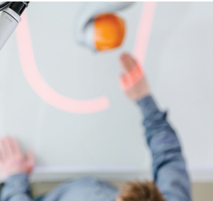
A robot stops immediately whenever the dynamically projected safety zone around it is breached.
