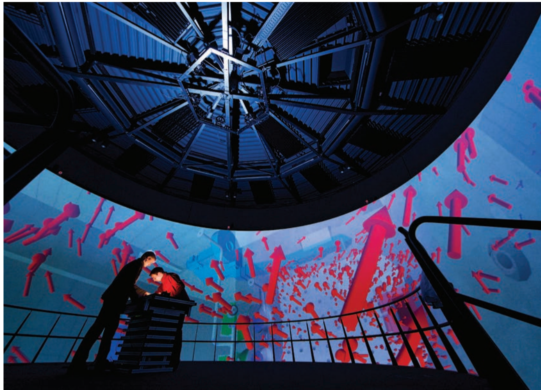
The “old” Elbe Dom with a 360-degree projection screen, a diameter of 16 meters and a height of 8.5 meters was one of the largest visualization systems for virtual interactive applications for business and research in Germany. Photo: Thomas Ernsting
