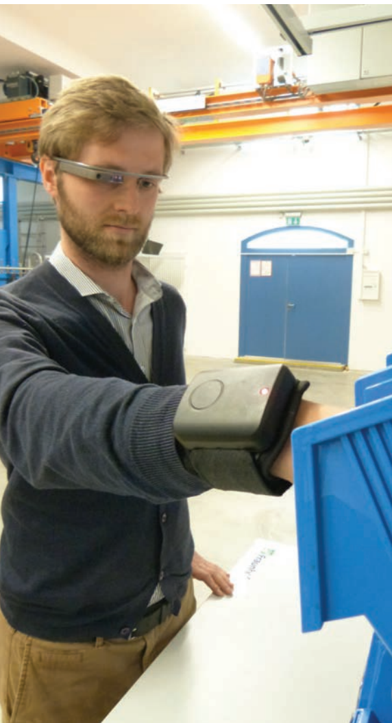
Testing the integrated system with RFID Wristband and Smart Glasses. Photo: Fraunhofer IFF
