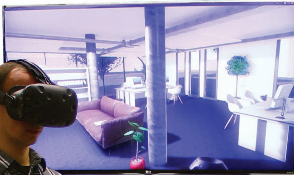
Virtual interactive inspection of planned construction projects conveys a very realistic impression of a future building. This is based on 3D data of a building. This makes it possible to review and assess options and alterations swiftly. Photo: Fraunhofer IFF
