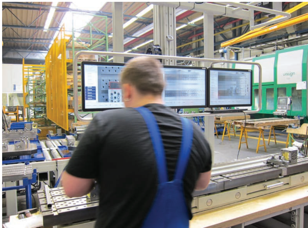
A "digital assistant" helps a worker assemble parts in a complex assembly such as the electrical enclosure here. The system shows the worker on a monitor how to assemble the part or whether there is an error. Photo: Kolbus GmbH & Co. KG
