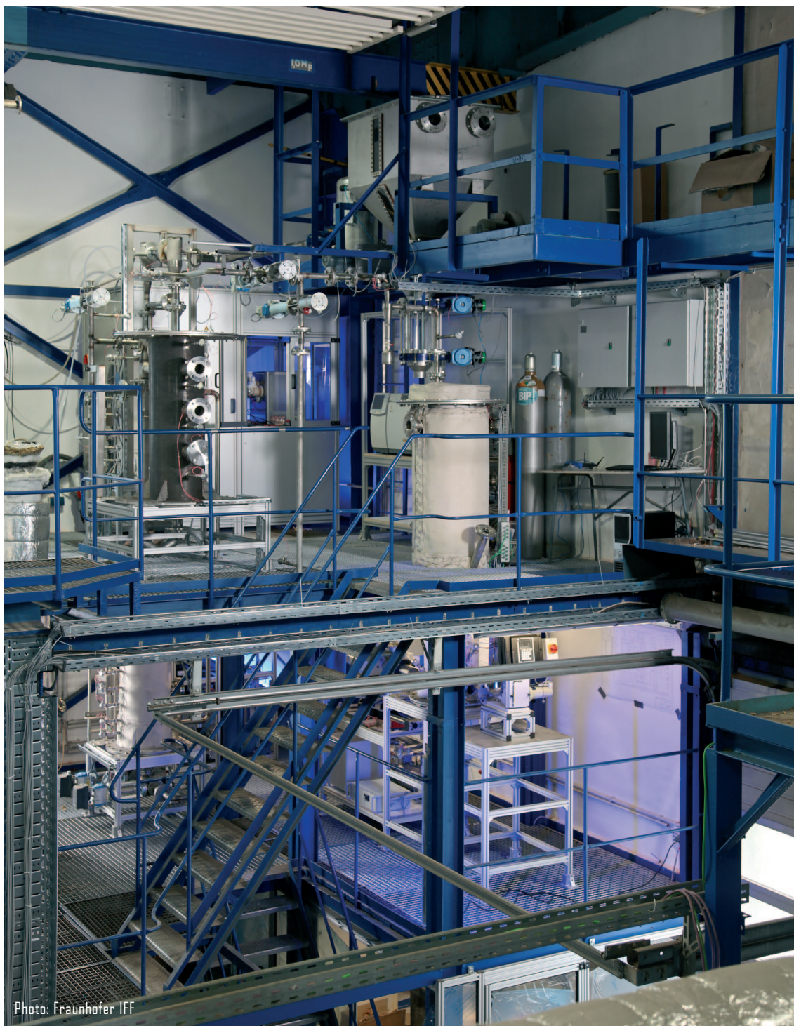
The test units in the fluidized bed testing facility. The Fraunhofer IFF uses them jointly with Otto von Guericke University Magdeburg for its tests.
