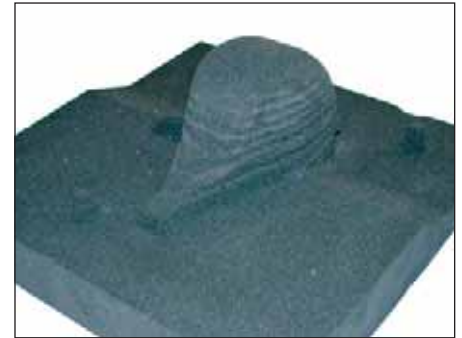
Fig. 2: Milled sand mold. Photo: Torsten Felsch
