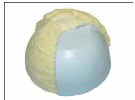
Fig. 3: Laminate model making combined with milling afterward. Photo: Torsten Felsch
