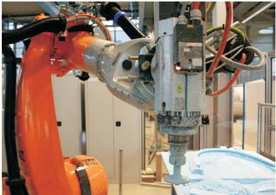
Fig. 1: Milling application with an industrial robot. Photo: Torsten Felsch
