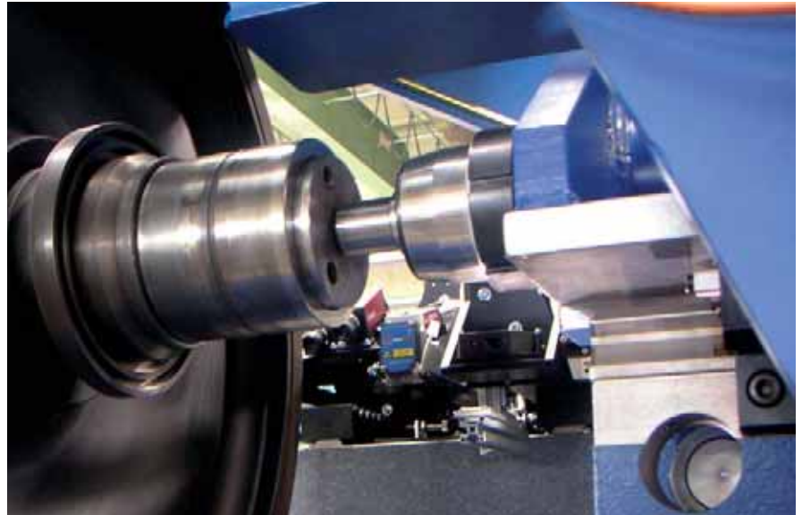
An optical 3-D measuring system inspects wheelset quality. Photo: Anna-Kristina Wassilew
