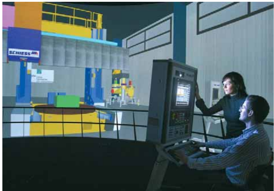
Fig.: A real CNC coupled with the virtual model of a heavy machine tool. Photo: Dirk Mahler
