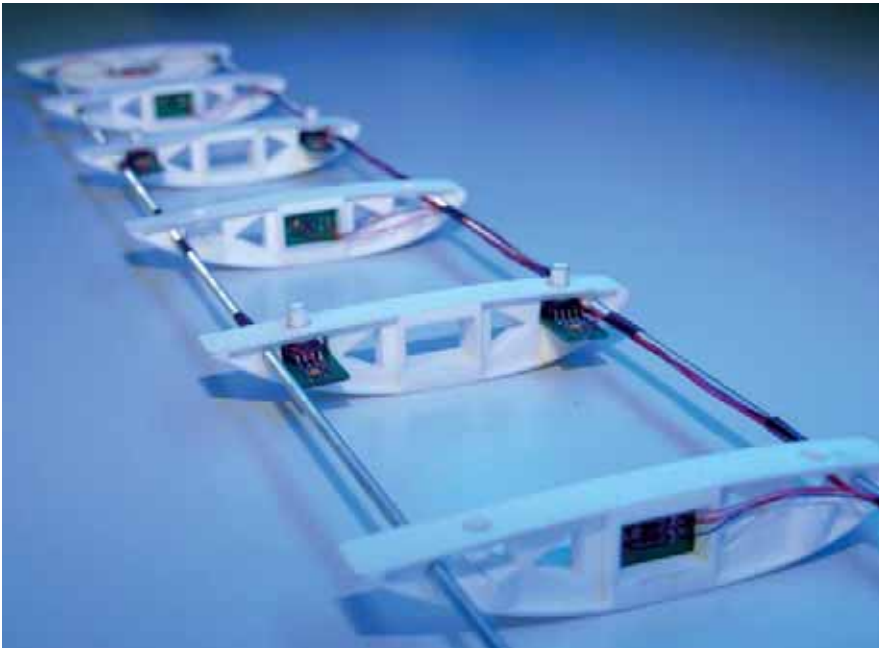
Major carmakers send their cars to race in the German Stock Car Championship (DTM). Researchers from the Fraunhofer IFF developed an intelligent rear spoiler for their industry partner TR Engineering. Sensitive sensors make it possible to actively influence aerodynamics so that the optimal ratio of downforce and drag can already be determined during test drives. Photo: Anna-Kristina Wassilew
