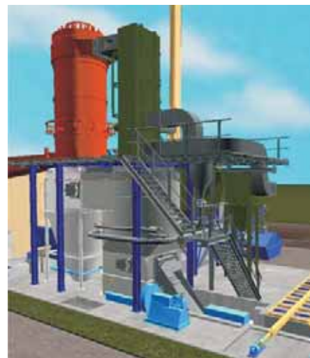
Fig. 3: 3-D representation of the firing plant (gray) with thermal oil boiler (red) and economizers (green).
