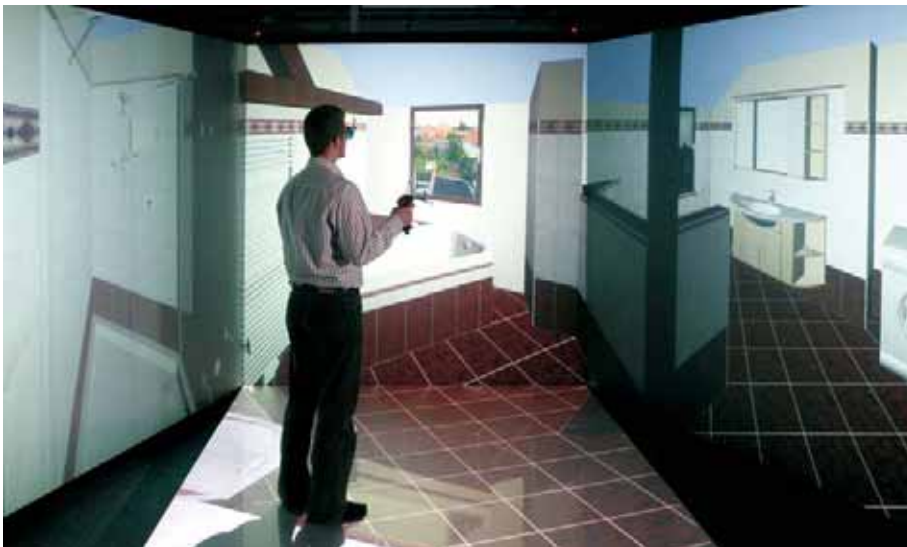
Fig.: Visualization of a bathroom design in an immersive multisided projection system (CAVE) at the Fraunhofer IFF. Photo: Dirk Mahler
