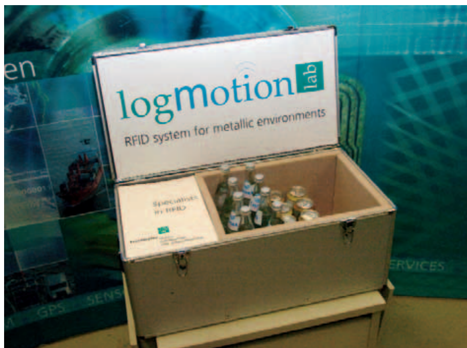
Figure: The Smart Metal Box functions reliably even in metallic environments and with such objects as metal cans filled with liquid.
