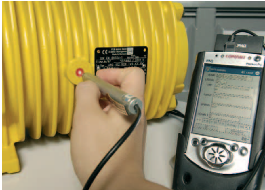
Figure: A handheld can be used to retrieve and update information directly on an object. (Photo: Siemens Press Foto)
