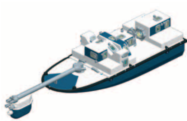
Figure 2: SEK damage detection unit for preliminary inspection of large sewer lines.
