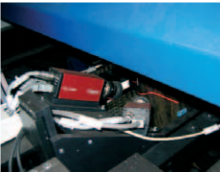
Figure 2: Optical sensor cluster that captures profile characteristics.
