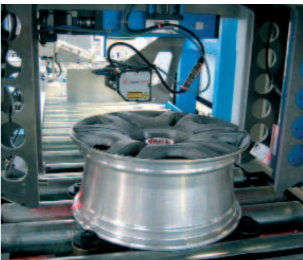
Figure 2: Automatic acquisition of wheel geometry data in the 3-D measuring machine.
