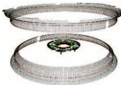
Figure 3: Digitized 3-D data of a wheel's bead seat and rim.
