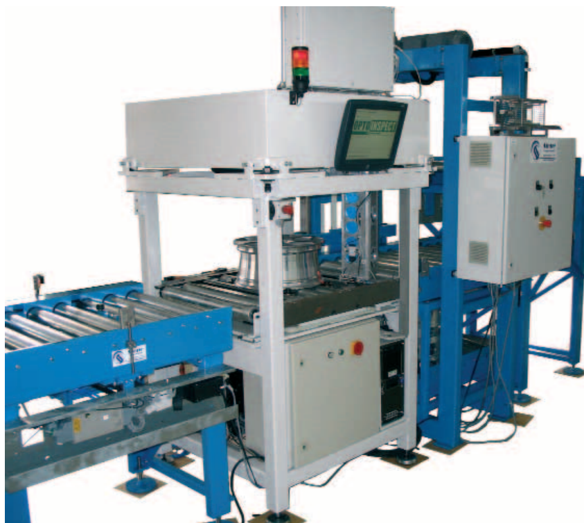
Figure 1: Measuring machine for in-line automobile wheel geometry inspection.
